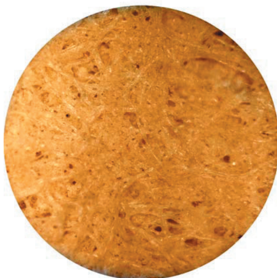
Microstructure of P202 50X
